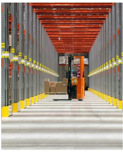
P90 Wide Aisle Pallet Racking provides your warehousing teams with unrestricted access to all your pallets at all times. The system delivers versatility and assembly as single- or double-depth racks.
