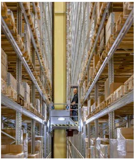
Crane racking is a dynamic, semi or fully automated warehouse solution. Its high density, high throughput is suitable for all storage types.
