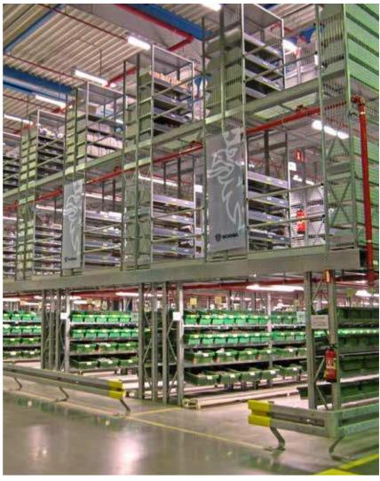
With Multi-tier Pallet Racking from Dexion, you can create manual pick-lanes for your teams at various levels, by providing walkways built into the pallet racking structure.
